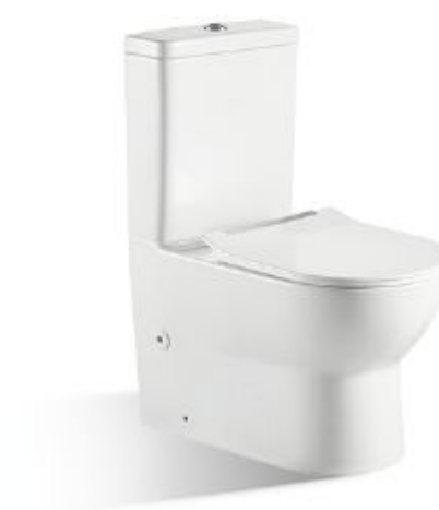
BL-116-TPT Washdown Flushing Toilet Size: 700×390×850mm P-trap: 180mm Roughing-in
